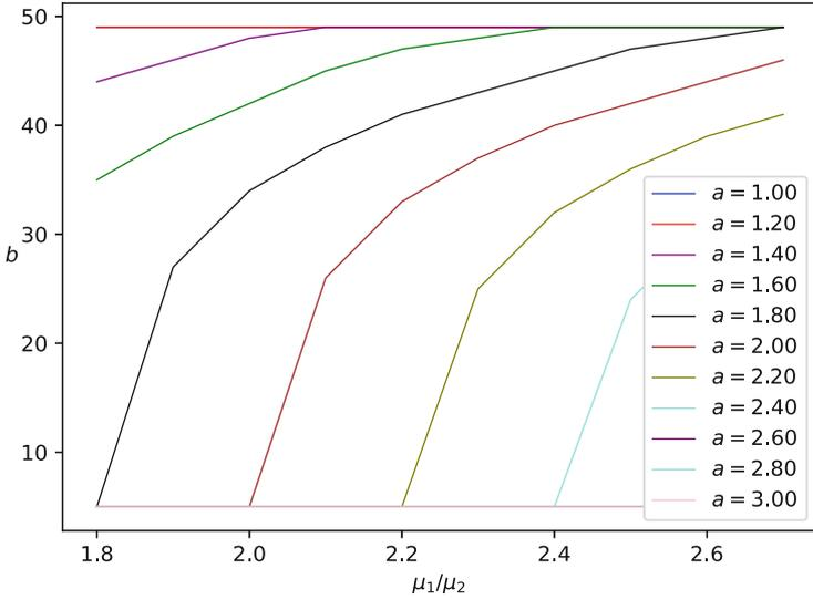
**Fig. 10.** The value of  $b$ , i.e. the energy level switching the performance of UAV from normal mode to energy saving mode, maximizing the reward function  $C(b)$  defined by Eq. (9) plotted as a function of  $\mu_1/\mu_2$ , where  $\mu_1$  is the speed of energy consumption in normal mode and  $\mu_2$  is the speed of energy consumption in energy saving mode, for fixed  $\mu_1 = 0.2$ .
