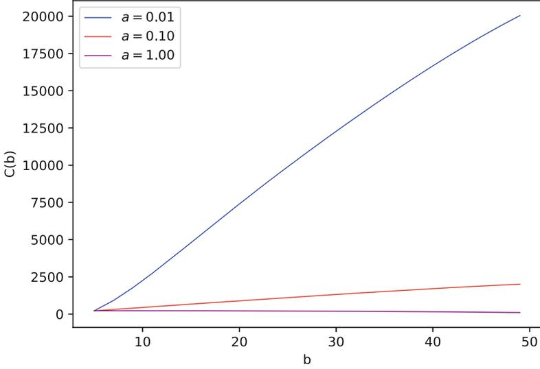
**Fig. 8.** The reward function  $C(b)$  defined by Eq. (9) and to be maximized;  $b$  is the energy level switching the performance of UAV from normal mode to energy saving mode, for linear function  $\Theta$  defining the decrease with time of the value of previously gathered data, see Eq. (11), with parameters  $\mu_2 = 0.10$ ,  $a = 0.01, 0.1, 1000$
