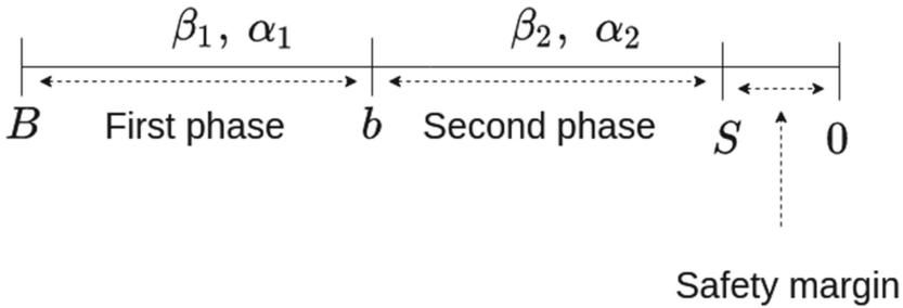
**Fig. 2.** The two phases of the UAV mission: in the first phase we assume that energy is used for flying, for ground communications and data acquisition. The second phase focuses on the landing phase, including any indispensable data acquisition and communications for the return to the landing base.
