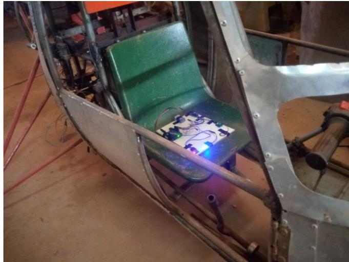
**Figure 12: Vibration detection Arduino module**
