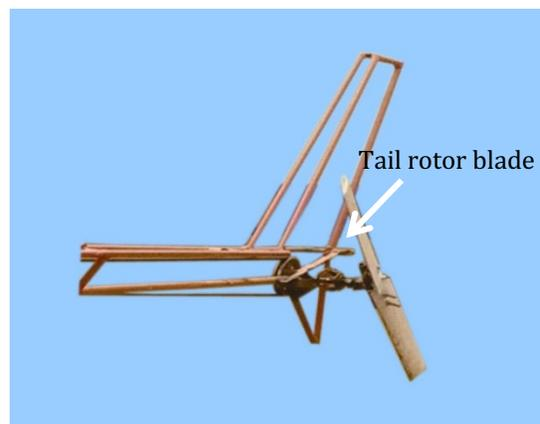
**Figure 4: Realized tail rotor**
