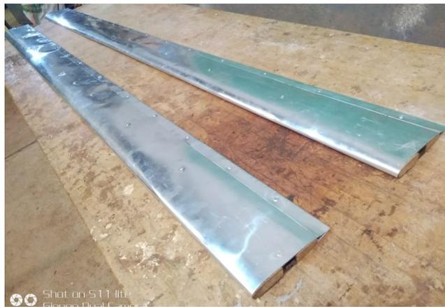
**B (b Rotor blades made of aluminum sheets)**
